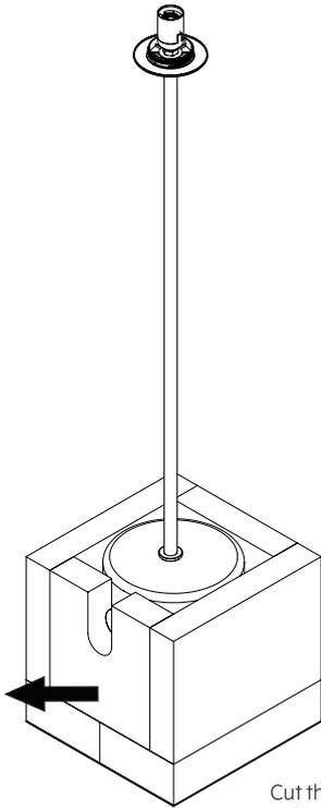
Cut the tape in the sides, and remove the part as shown.
