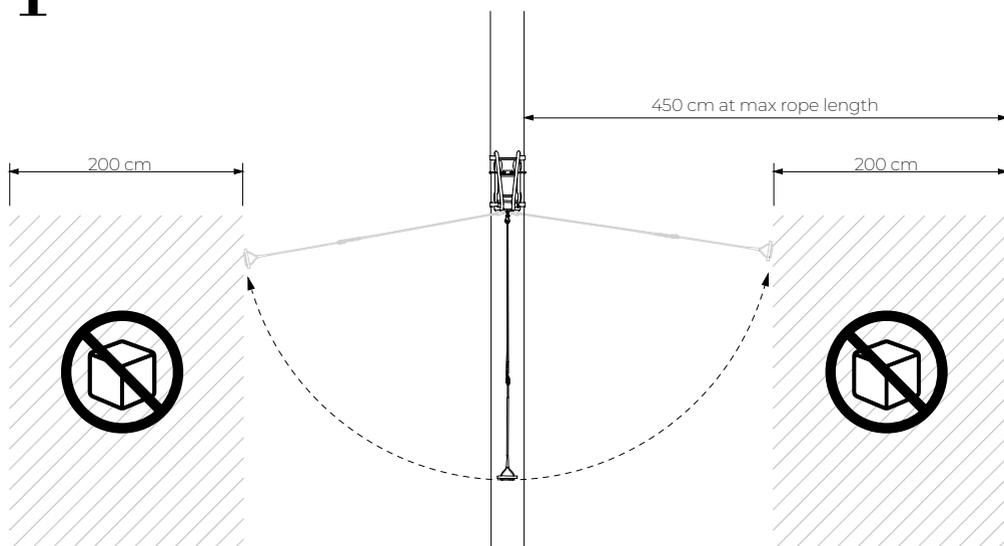
ENG Ensure a sufficient safety distance (at least 2m) from any obstacles (walls, fences, trees) in the direction of swinging.
