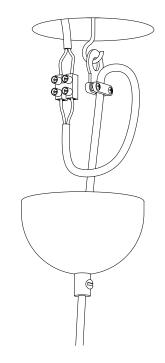
5. Control cable's length by unscrewing the cable grip screw and sliding the cable through. Restore power at the fuse box. Your product is now ready to use.
