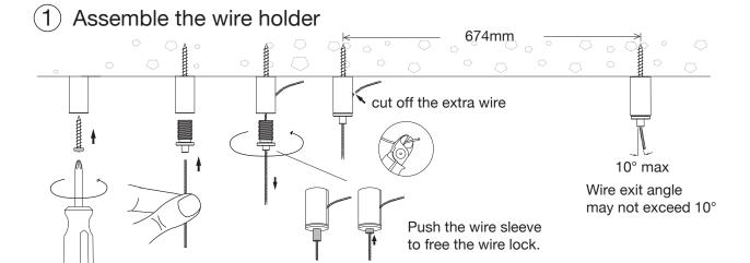
Be sure to insert the wire into the holder at least far enough to be able to clearly see it protrude from theother end of the holder. When attaching the holder into concrete or stone, use a screw anchor.
