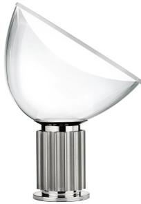
Table lamp providing indirect and reflected light. Reflector in painted aluminium, gloss white on the outside and matt white on the inside. Directionable diffuser in transparent blown glass. Body in matt black or naturally anodized extruded aluminium. Base in nickel-plated ABS+PC. Electric cable of useful length 190 cm, with dimmer switch for ON/OFF and adjustment of the light flow between 10-100%. Plug-in power supply with interchangeable plugs.
