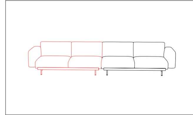
Starting from one side/end of the frame section, attach the individual modules loosely without leaving any gap in between.
