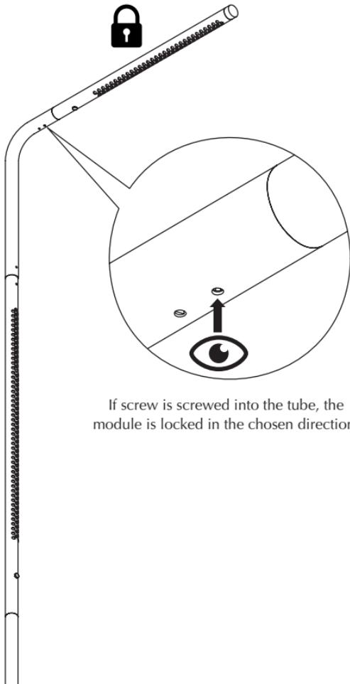
If screw is screwed into the tube, the module is locked in the chosen direction.
