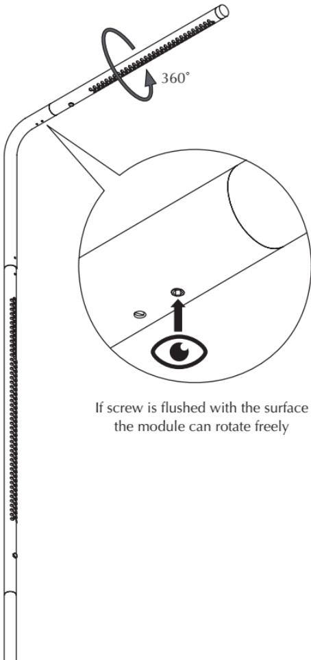
If screw is flushed with the surface
