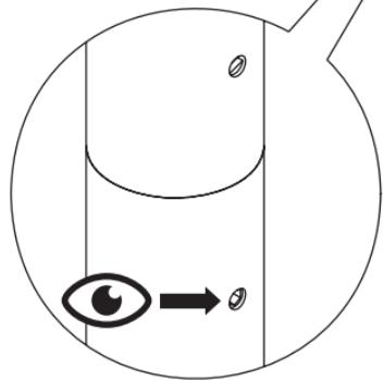
If screw is screwed into the tube, the module is locked in the chosen direction
