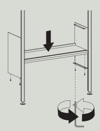
**OPTIONAL:** In case your configuration contains an additional cabinet shelf (H), slide it in between the two side panels from the top.
