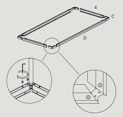
NB! Make sure the holes on the corner (C) are facing up.
