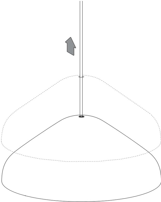
Adjust the height of the shade by screwing the plastic adjuster until the bottom edge of the shade and the diffuser are aligned. Screw it clockwise to lower the shade and counterclockwise to lift the shade.
