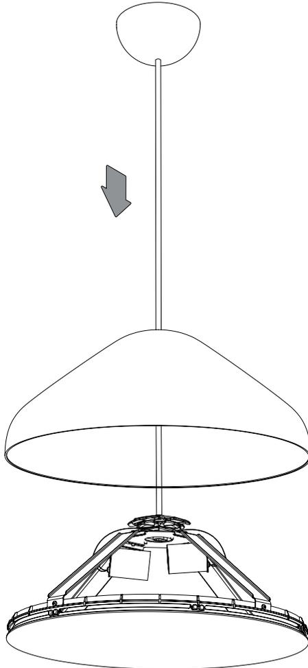
If the diffuser is visible underneath the shade (fig. 1) or the diffuser is too far inside (fig. 2), the shade can be adjusted so that the shade and diffuser are aligned.
