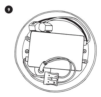
**I 0** Connect the wires to the two terminal clamps and pay attention that the polarity is correct. **Important:** The red wire must be connected to the terminal clamp on the red lead, and the black wire to the terminal on the black lead!
