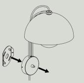
**Step 7** Carefully remove the lamp from wall bracket.
