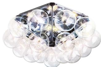
Wall/ceiling lamp providing direct and reflected light. Structure formed by 5 pressed polished aluminum triangles. 15 clear Globolux lamps housed around the structure. Steel wall/ceiling fitting and rose.
